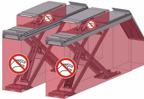
Fig. 3-1 Mechanical danger zones
